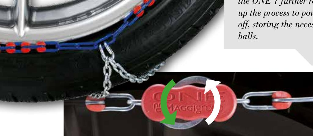
The special device supplies with the ONE SUV and the ONE 7 further recovers the clearances and speeds up the process to power the device when the vehicle is off, storing the necessary energy for running, in the balls.
