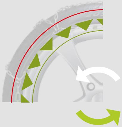
When the vehicle starts moving the system partially discharges the energy potentially stored, the deformed ball return to the original shape and the chain shortens along the circumference (green line).
