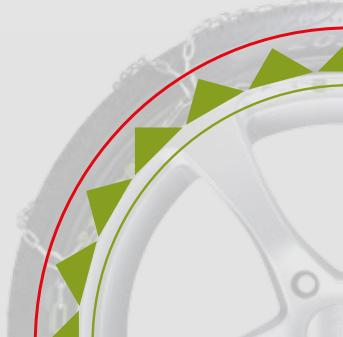
During assembly under voltage with the vehicle off - the system is charged with potential energy through the compression of the ball - the chain stretches along the circumference (red line).
