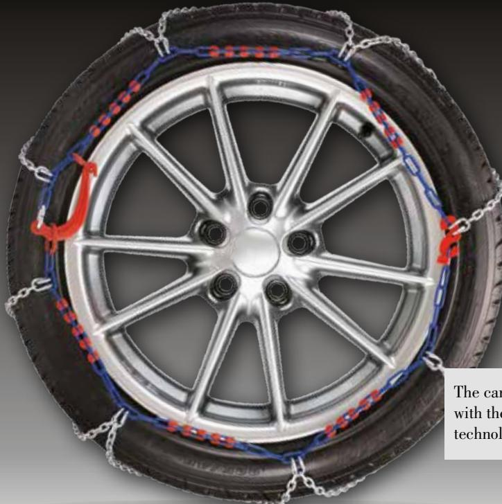
The car chain with 9 mm encumbrance with the revolutionary tensioning technology with elastomers.
