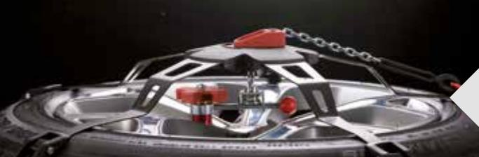
*The combined action of the force applied across the rubber, generated by the arms and by the centrifugal force applied to the moving tyre, automatically moves the chain to the most suitable position.*
