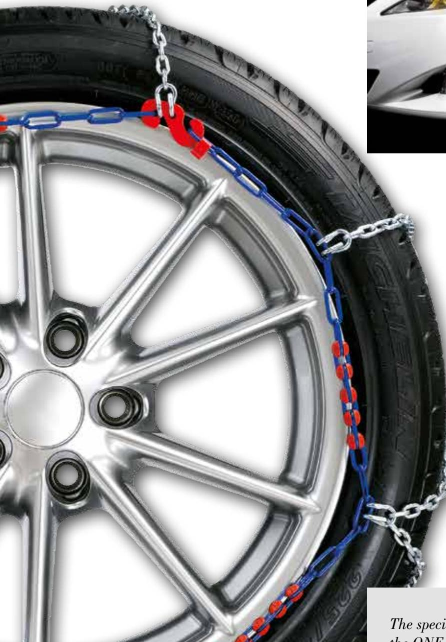
The lever fastening device helps locking the chain during installation, thanks to the special ergonomic shape.
