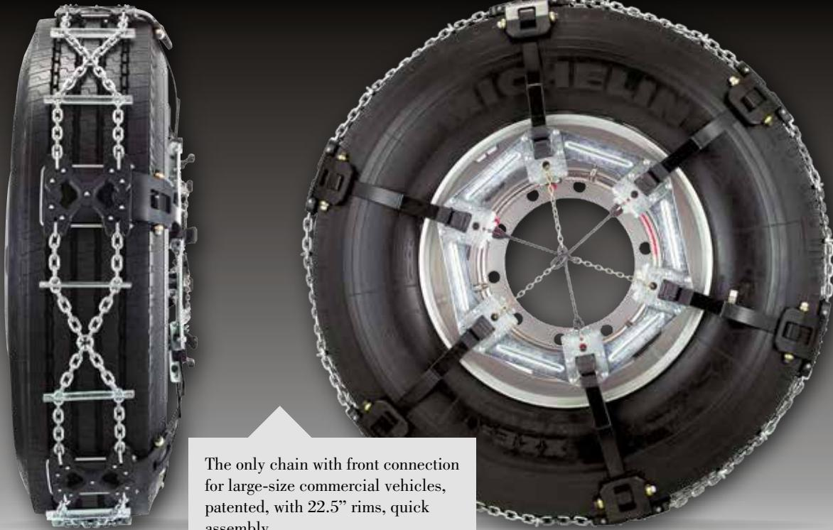
The only chain with front connection for large-size commercial vehicles, patented, with 22.5" rims, quick assembly.
